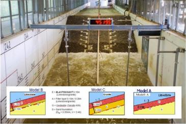
Fig.1 Large Wave Flume (GWK), Hannover. Breaking wave on PBA revetment
