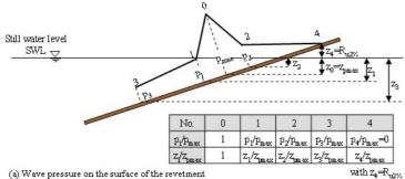
(a) Wave pressure on the surface of the revetment
