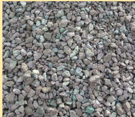
Aggregate from recycled Shell Thiocrete products.
