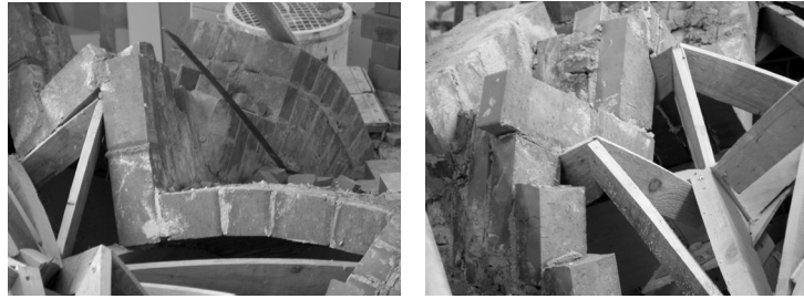
Figure 2: Experimental reconstruction of a cell vault at Trebsen, 2005. The centering of the re-entrant groins is subject to discussion, as it is conflicts with the preliminary analysis (Förderverein für Handwerk und Denkmalpflege e.V. – Schloss Trebsen).
