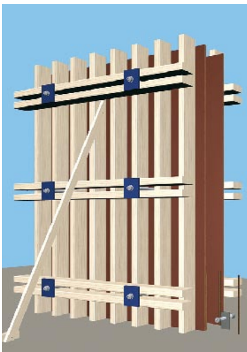
A Traditionele wandbekisting
