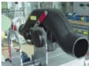
1. Fix fitting in welding machine
